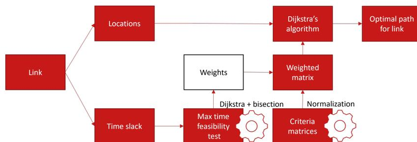
Figure 11: Visualization of model CurrLink: link analysis
